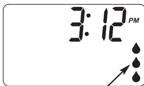
Droplets indicate water flow through conditioner
