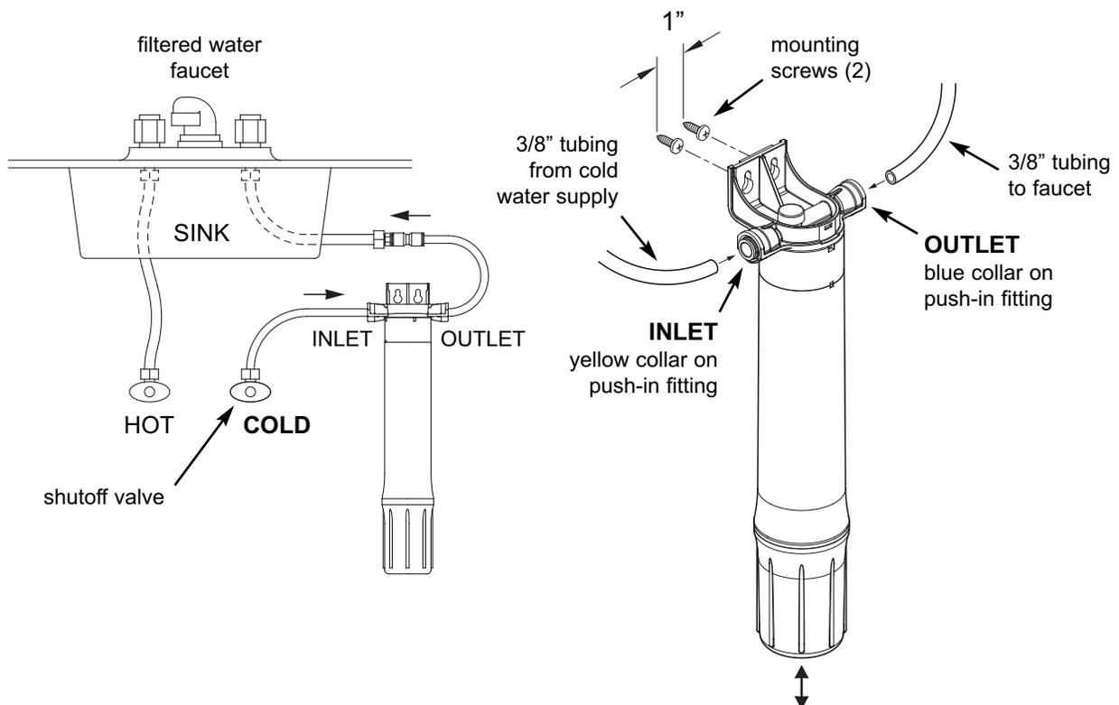
**NOTE:** Be sure to allow a minimum space of 1-1/2" under the system for removing the filter cartridge to change it.
